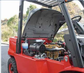
The enlarged opening angle of hood and increase of left and right hood side plates can provide you with convenient and rapid maintenance mode.
